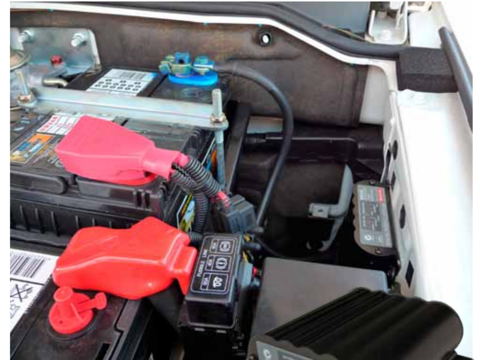
BCDC1220 installed in a Pajero NT 2010 model
